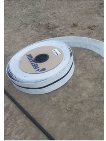
Figure 19. Layflat header hose ready for rolling out.
