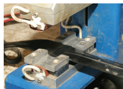
Figure 57. Splicer to repair dripline for re-use. Photo by M. Cahn.
