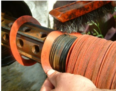
Figure 49. Check and clean filters.
