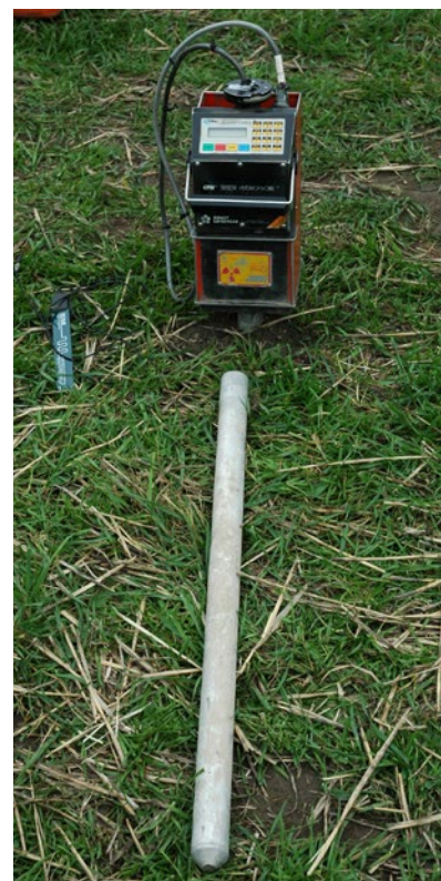
Figure 51. A Neutron Probe gives accurate measurement of soil moisture.
