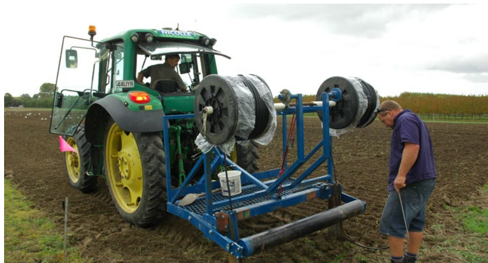
Figure 35. Laying machine set to place two rows of dripline at 1.5m centres.
