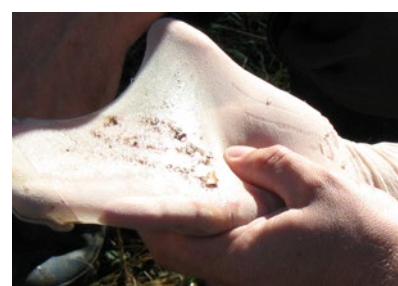
Figure 47. Checking water from a lateral for presence of contaminants or debris.
