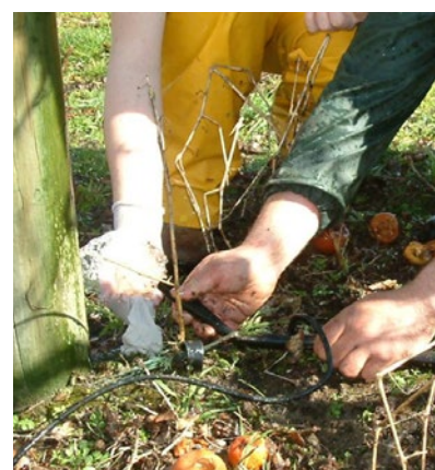
Figure 46. Strain flushing water through a stocking to determine what contaminants are present.
