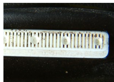
Figure 45. Fine sand particles collecting inside emitter.
