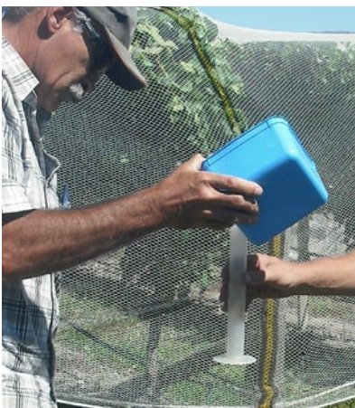
Figure 43. Measure individual emitter flows at key points.
