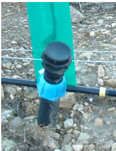
Figure 34. Flushing point for permanent drip in a vineyard.
