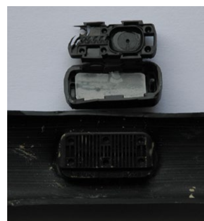
Figure 15. Inside of compensating emitter: bottom, the strainer; centre, inside of emitter showing rubber diaphragm and top, flow path and outlet.
