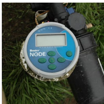
Figure 27. Simple time-based battery-operated in-field zone controller.
