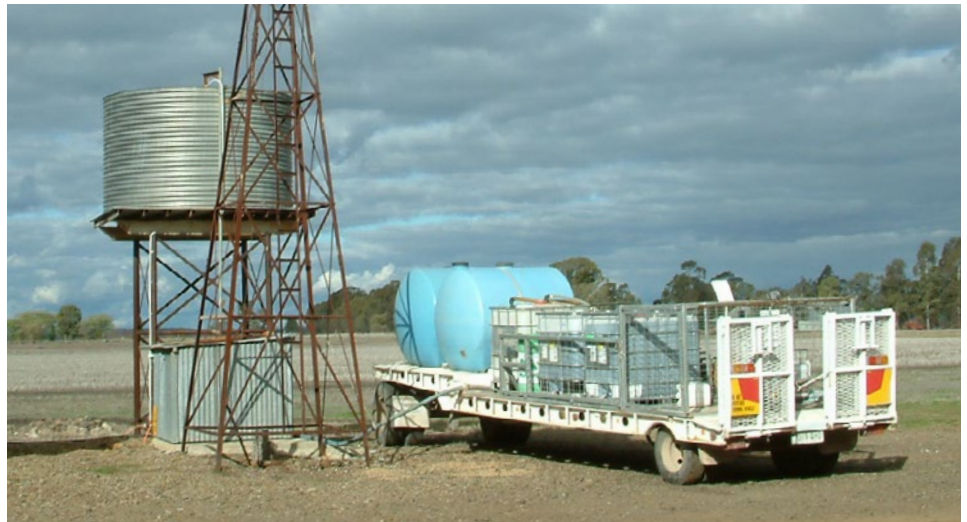
Figure 54. Mobile fertigation rig with concentrates in separate containers.
