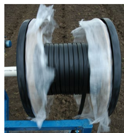
Figure 38. Dripline is wound off the spool and through a shank into the ground. Care to avoid sharp points on equipment is essential.
