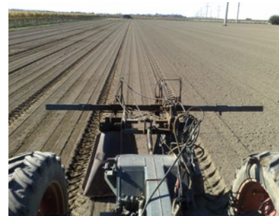
Figure 8. Scott's tractors auto-steer with centimetre accuracy, a real advantage with buried drip systems.
